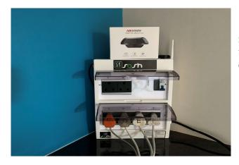
**SASH Controller:** Plug in up to 6 devices to control, temperature and humidity sensor and an auto focusing camera: **SASH**.
